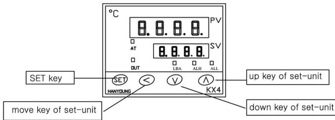
When you power on the controller, PV shows current room temperature and SV shows set temperature. Recommendation is 250°C~350°C. After turn-on & set, within 10 minutes, it reaches to set temperature.
