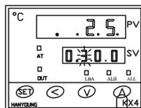
③ Set desirous temperature by pressing up and down keys.(i.e :300°C). Set-temperature will be increased by up key and it will decreased by down key.
