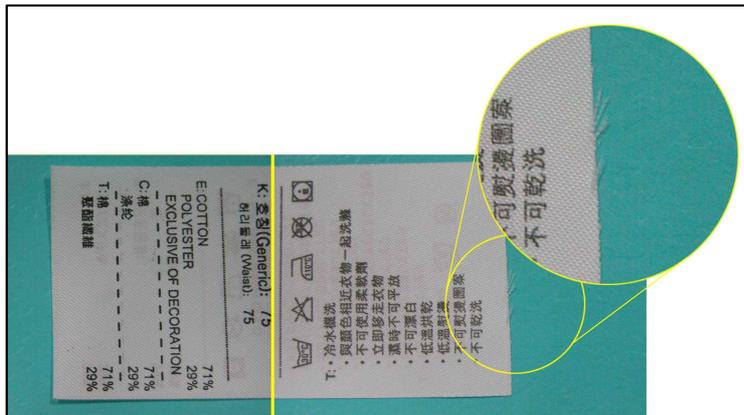
Sometimes you can see a label, one side is sealed well, but the other side is not sealed well.
