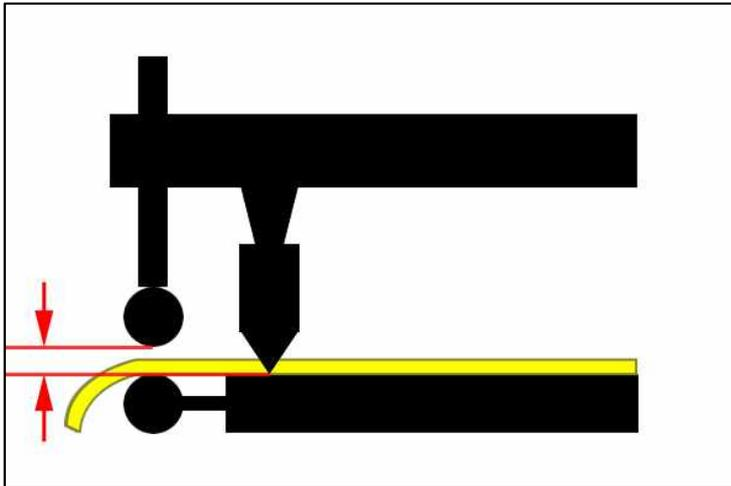
As you can see left image, the upper front feeding roller is higher than hot-knife.
