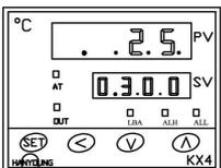
④ After finishing setting, press SET key once more. Then, it stops blinking. And the controller will return to auto-tuning mode.
