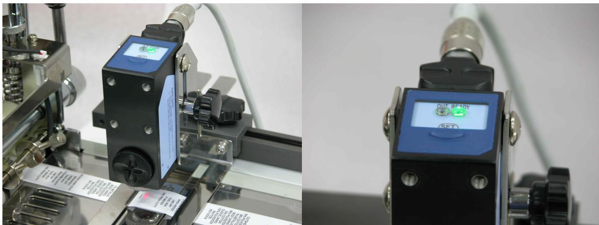
⑥ By moving sensor, make sensor light indicate cutting mark again.
