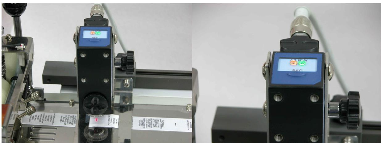
If you did it correctly, when you make sensor light indicate cutting line, the "out" lamp is on.
