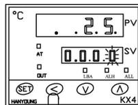
② By pressing left key, you can move between numbers of four ciphers. as follows.
