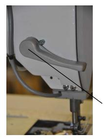
Turn the lever 1 downwards. The presser feet are locked in their utmost upper position. Turn the lever 1 upwards. The presser feet are released. Or Lift the presser feet pneumaticaly by the foot pedal or mechanically by the knee lever . The lever 1 will turn back to its initial position.
