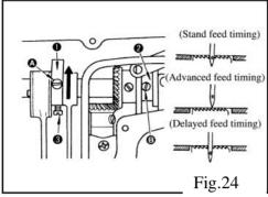
1)To obtain the standard feed timing align setscrew@on feed eccentric cam①with setscrew@on main shaft thrust collar②. 2)To make adjustment,loosen two setscrews③to release the feed eccentric cam,properly position the eccentric cam. Then retighten the setscrews.
