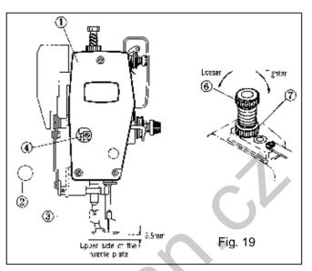
weaker when turned counterclockwise. Make sure to screw in the fixing nut (1) after adjustment. (Fig.19)
