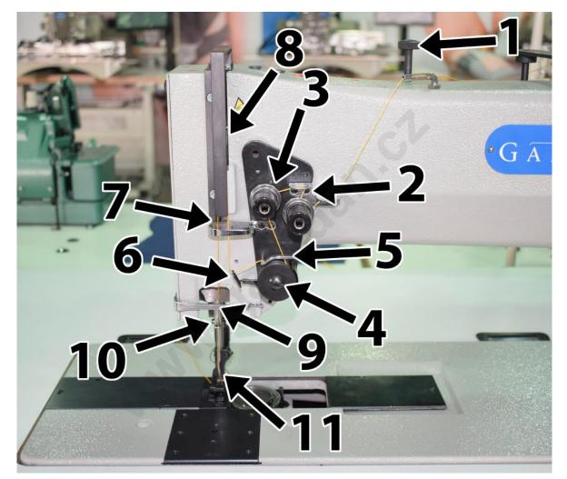
2. With the left hand hold the end of the needle thread leaving it slack from the hand to the needle. Turn the machine pulley over toward you until the needle moves down and up again to its highest point, thus catching the bobbin thread, draw up the needle thread, and the bobbin thread will come up with it through the hole in the feed dog. Lay the threads back under the presser feet and close the slide.
