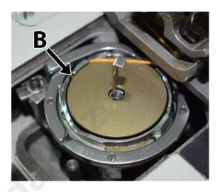
To increase the tension turn the nut or screw clockwise, and to decrease the tension turn the nut or screw counter-clockwise.
