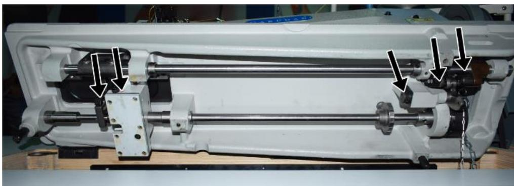
2. To fill the oil for hook saddle reservoir: take out the oil gauge from the hole (A) pour the oil into the hole until the oil level reaches the upper reference line of the oil gage (B).
