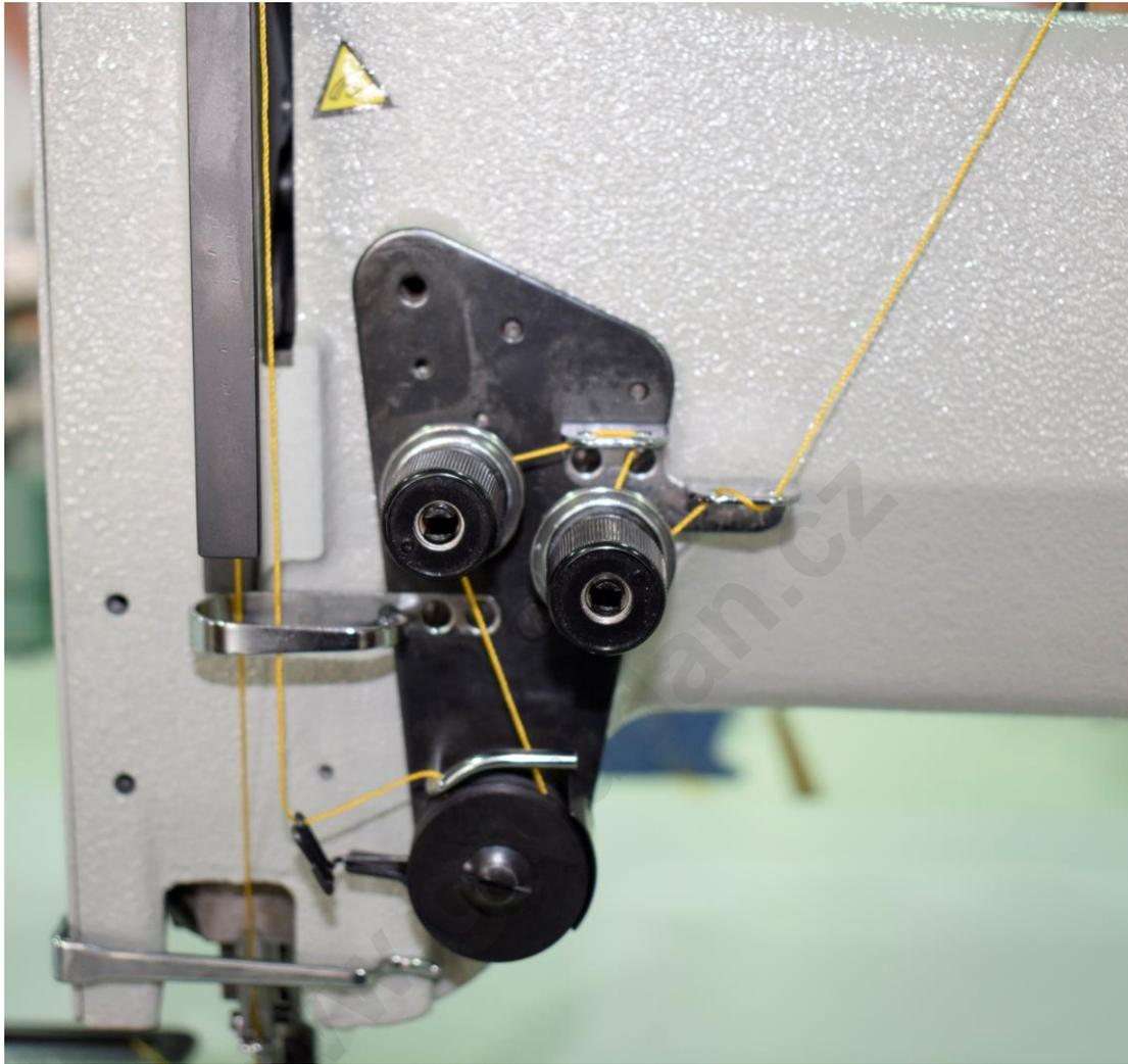
Threading detail for twin-needle machine:
