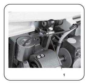
• Adjustment of feed dog (3) height against the needle plate (4). Turn the main shaft to 190°, loosen the screw (1), adjust the feed dog (3) to be 0,5mm higher than the needle plate (4),tighten the screw (1).
