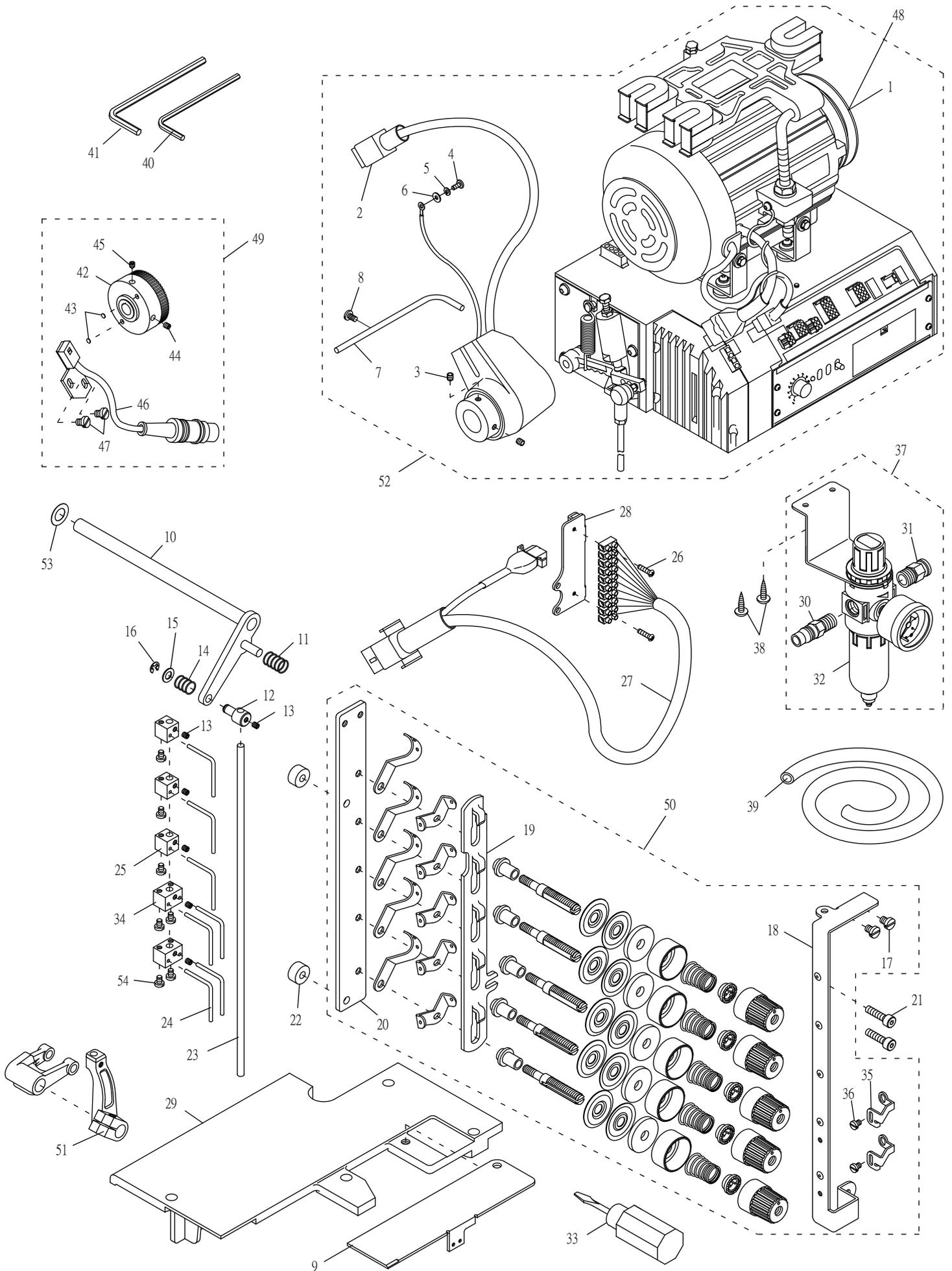
4. PA 鬆線機構及更換零件 PA Thread Tension Components And Motor Components
